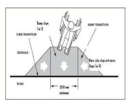
Curb ramps shall have a minimum width of not less 1 200 mm in areas measured across the ramp. The sides of the curb ramp shall be flared. The gradients of the curb ramp shall be 1 in 12 and the flared sides shall be not more than 1 in 10. Curb ramps should have a surface that is slip-resistant, and colour and texture contrasted with the adjacent surfaces.
